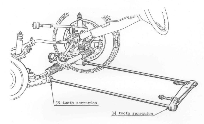
Suspension height is adjusted by rotating the torsion bars.
