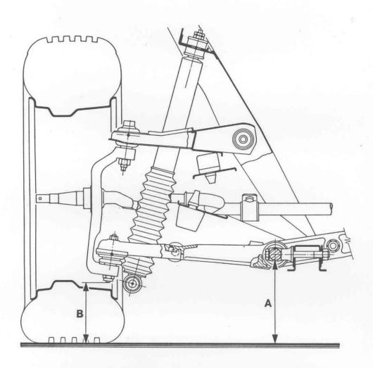
Dimension "A" must be measured in correspondence of the lower line of wishbone shaft as shown.
