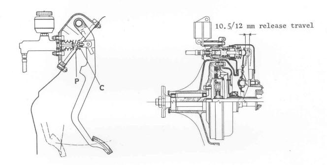
If necessary, check that, when the clutch pedal is depressed fully the push rod of slave cylinder moves through a total travel of 10.5 to 12 mm.
