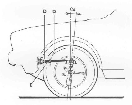
The difference in caster angle between R.H. and L.H. wheel must not exceed 0° 201.
